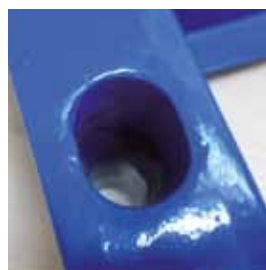
Original anchor sleeve – oval cone with offset radii
