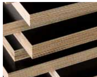
Formwork sheet – laminated plywood 18 mm (class 1/1). Face-film thickness – 220 g/m 2
